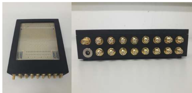
Figure 8 26 GHz mmWave frontend
