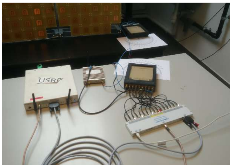
Figure 16 User side USRP with RF switch and 26GHz antenna array.
