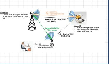
This showcase demonstrates the fast beam steering algorithm of TUD. Under the mobility scenario, the system is able to successfully track the best beam pair with a maximum delay of 20ms and minimum delay of 2.5 ms when the best TX beam changes by one beam. In addition, the capacity of the mmWave frequency band is duplicated by reusing a second link with. Additionally, we demonstrate the employment of two sub 6 GHz links operating in TDMA mode.
