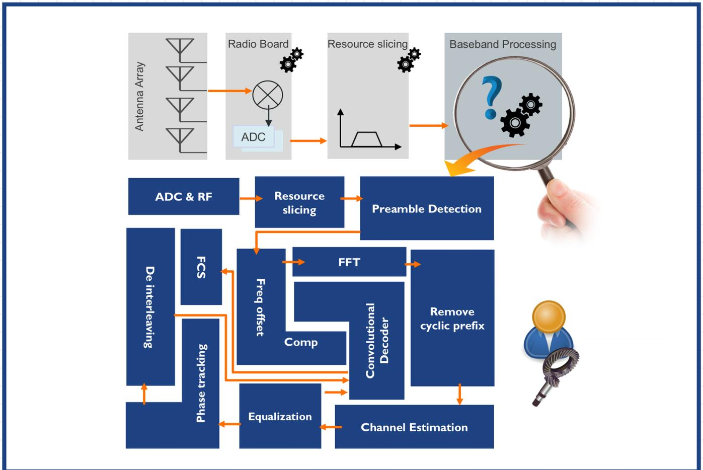
→ Signal processing chains are divided into micro blocks, such as preamble detection, symbol-level processing, bit-level processing blocks and etc.
