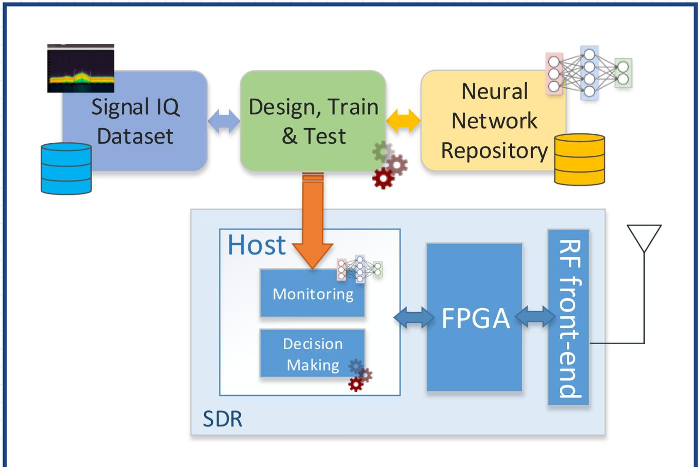
Spectrum monitoring prototyping platform for experiments on RAT identification and parameter estimation
