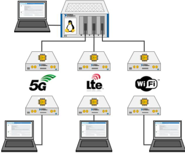
Fig. 2. Realization of the multi-RAT platform with SDR hardware
