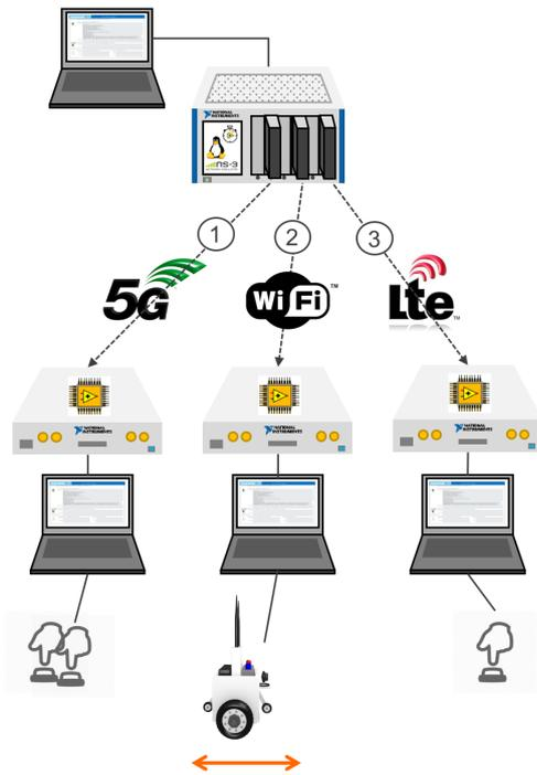
1. Either of the two buttons connected to the 5G or LTE link can be used to control the moving direction of the robot
