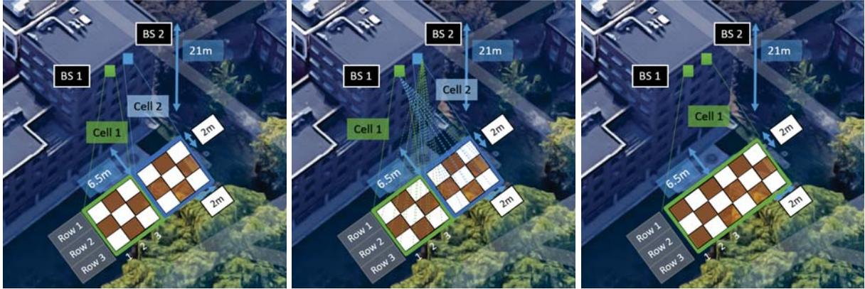
(a) Two-cells scenario: Each cell operates in a different band centered on different carrier frequency without interference. (b) Spectrum sharing scenario: Both cells operates in the same band without coordinated spectrum sharing. (c) Infrastructure and spectrum sharing scenario: Two coordinated BSs serve all UEs in the system, using the same band.
