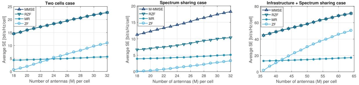
(a) The average SE per cell in a system with two independent cells, that operate on different carrier frequencies. (b) The average SE per cell in a two-cell system with a shared carrier frequency and two networks share spectrum and infrastructure. (c) SE in a system with distributed BS, where two networks share spectrum and infrastructure.
